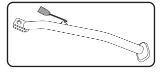
4. Install (No. 12/13) 11660-BRKT-L/R, left and right muffler hanger brackets where passenger footpegs where removed using (No. 5) M8X20, bolts and (No. 7) 8MMNUT, nuts. See diagram for proper orientation and order of hardware. Do not torque at this time.
