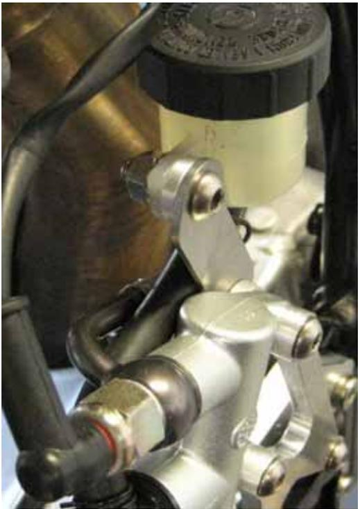
Fix reservoir and spacer (t=4mm) on the bracket's inside with M6x18. Mount washer and locknut M6 from behind.
