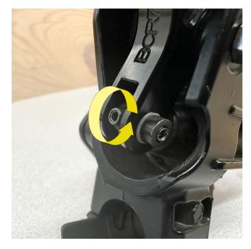
4c) Use the 2mm hex key wrench to tighten the push rod retainer screw until the colored threads are no longer visible or flush.
