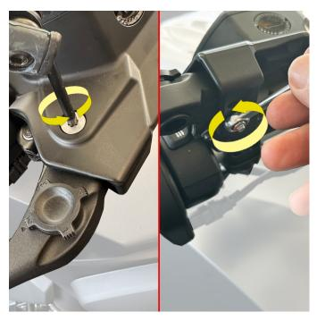
3b) Once the nut is off, use your fingers or a flathead screwdriver to push or pull the Torx bolt out of the master cylinder. Carefully remove the lever from the master cylinder.
