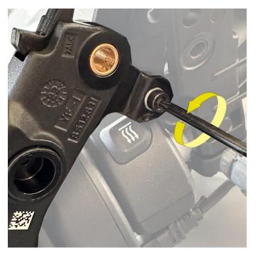
3d) On the inside of the lever, use the 2mm hex key wrench and turn the push rod CLOCKWISE until you hear a clicking sound. While turning, make sure you don't dislodge the rubber retaining boot.
