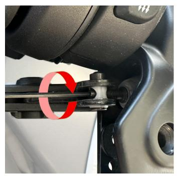
3e) Retain the push rod barrel. It will be needed for the ASV lever.
