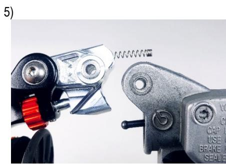
5) Insert the **RETURN SPRING** into the ASV lever. Do not reinstall the black rod.
