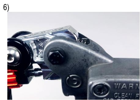
6) Insert the ASV lever into the stock perch and insert the pivot bolt. Screw the bottom nut until secure.
