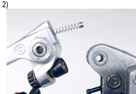
2) While removing the pivot bolt, hold the **RETURN SPRING** as it will pop out when the lever is free. Remove the black rod from inside the spring.
