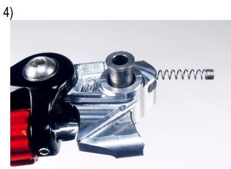
4) Insert the **STOCK BUSHING** with the rim side up into the ASV lever.
