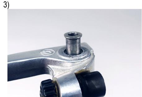
3) Remove the **STOCK BUSHING** (metal sleeve) from the stock lever.
