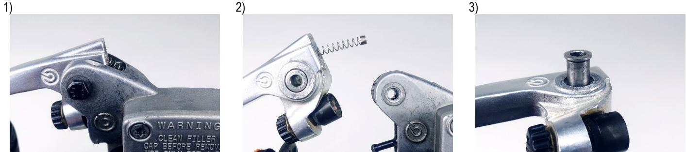
1) Unscrew the bottom nut and remove the pivot bolt.
