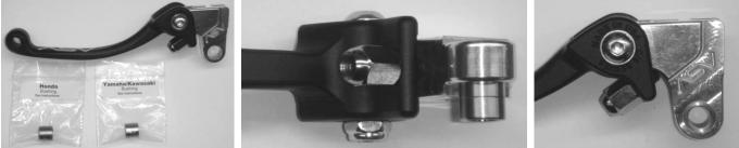
3. Complete installation using the stock bolt and locknut. The lever should fit snugly but move freely, just like the stock lever. If the lever is too loose in the perch or the bolt does not fit, verify that the correct bushing has been selected.
