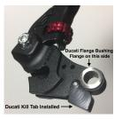
Follow steps 5–7 on the instruction card for installing your ASV clutch lever onto the perch of your motorcycle.
